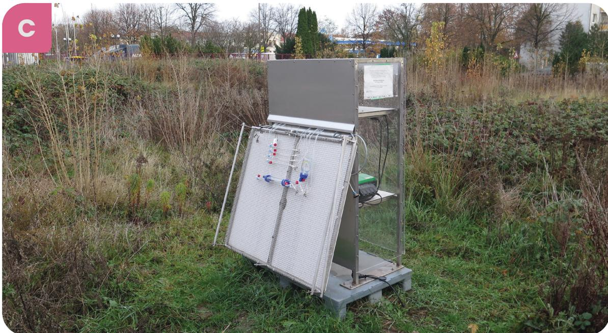
Capillary biofilm reactor in the lab (A) and outside running under real-world conditions (C). (B) shows example graphs from flow cytometry allowing close monitoring of population dynamics in the reactor.
