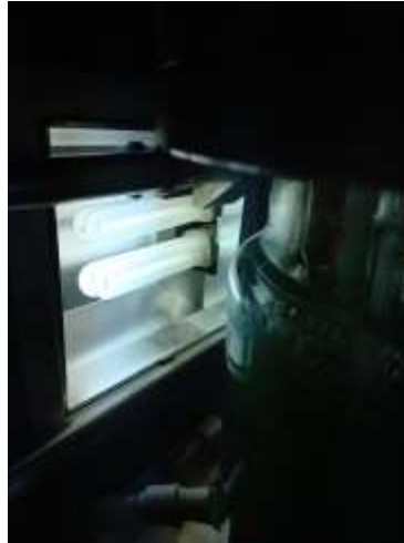
Figure 7. Fluorescent lamp used on the DC-PBR. The source of light are two fluorescent lamps on each side of the bioreactor. Each lamp carries two bulbs. The light shutter was closed to allow the visualization of the device.
